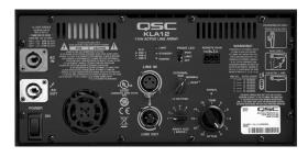
In an installed application, multiple KLA Series loudspeakers can be "daisy-chained" for total gain control from a single remote pot wired to the on-board Phoenix-style connector. Additional power module characteristics on KLA include a balanced, line-level XLR input in parallel with an XLR "Thru" connector, powerCON® In and Thru connectors, Attenuation Control and LED indicators for Signal and Limit, as well as discrete LED indicators for Power/Standby status.
